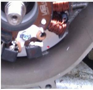
The base plate has - somewhat to the left of the 2 smaller black coils - a small red dot which indicates the ignition marking.
