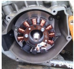
Place the new stator base onto the engine block. Fasten the plate with the base plate screws (please use the supplied ones, they need to be fairly flat).
