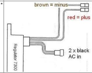
The new regulator/rectifier has 4 wires
